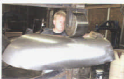
10) After more wheeling, the shape pattern fits the panel tightly. The panels are fit to the buck, as this helps ensure proper alignment for welding the two halves together.
