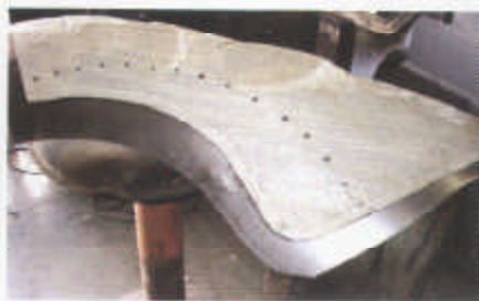
9) A quick check for fit to the shape pattern reveals there is more shaping to do. This is done through a combination of stretching and shrinking.
