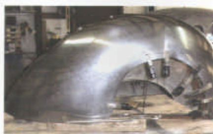
11) From this angle, you can see that the fender is securely fastened to the buck. These are in the proper location for mounting the fender to the body.
